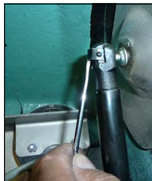
Fig. 10-9 Using a screwdriver, lift the clips and loosen the springs
