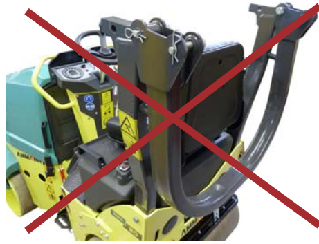
Fig. 3-2 Never fold the ROPS down during operation
