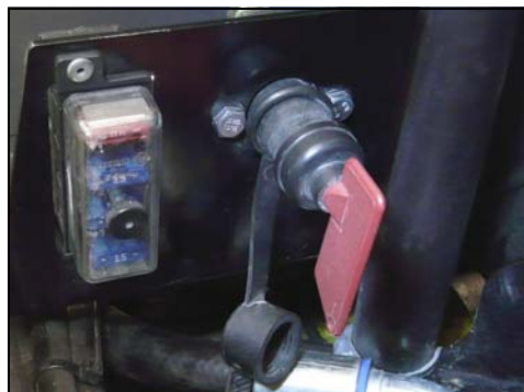
Fig. 8-8 Switching off the power
