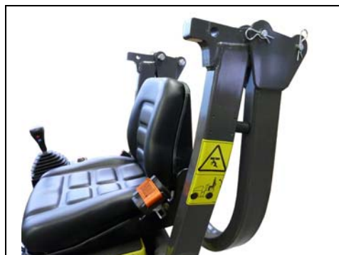
Fig. 7-1 ROPS down / ROPS up
