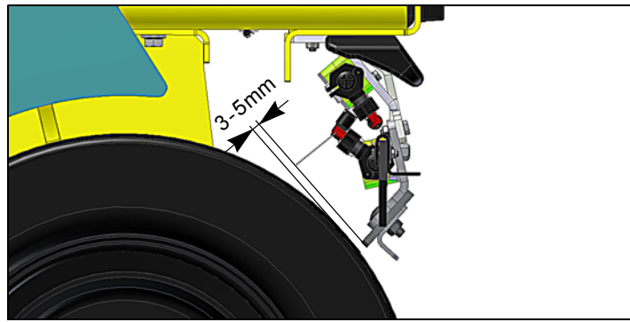
Fig. 9-24 Clearance of scraper to pneumatic wheels
