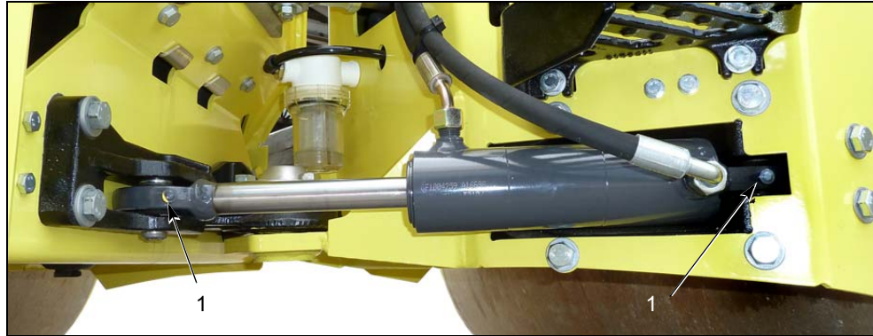
Fig. 9-32 Location of grease nipples on steering cylinder
