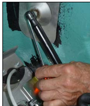
Fig. 10-9 Using a screwdriver, lift the clips and loosen the springs
